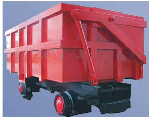
Apparatus for transporting materials is made in a form of wagons, WAGONS with manual filling arc made from 0.8 to 10 m<sup>3</sup>, and for tracks 0,6; 0,7 and 0,76 m, with one-sided tipping using a special machine or hydro. Wagons are very durable, robust, cost effective and very safe in production.
