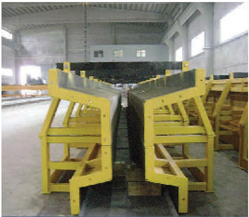
**STEEL FORMWORK** for concrete is used for building road tunnels, railway tunnels, hydro tunnels, underground halls, underground facilities etc. They are made according to our own project documentation or a clients documentation.
